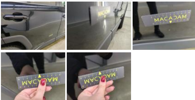
Door FR, Scratch(es), Repair and paint (complete)
