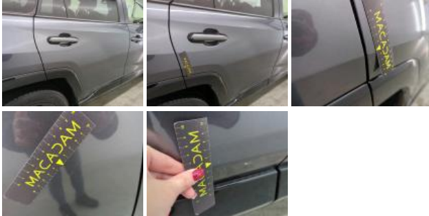
Wing RR, Dent(s), Repair and paint (complete)
