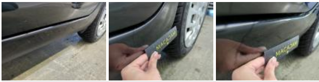
Door RL, Scratch(es), Repair and paint (complete)
