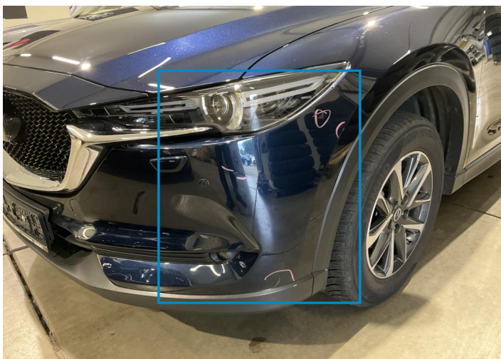
1. Corner Bumper / Front Left Bodywork / Dent / Dent -
