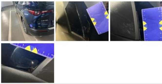
Bumper moulding R, Scratch(es), Smart repair
