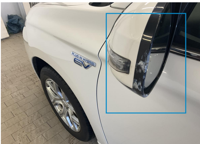
2. Mirror / Front Left Bodywork / Breakage / Crack -
