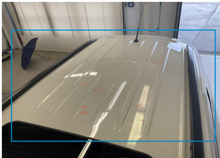
5. Roof Bodywork / Dent / Dent -
