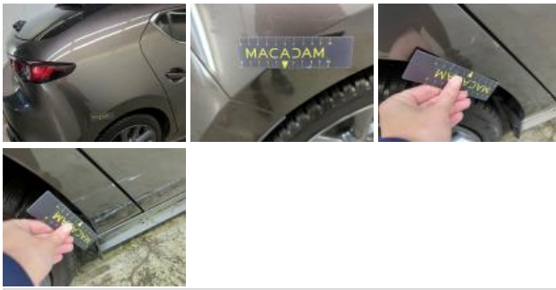
Door RR, Scratch(es), Repair and paint (complete)
