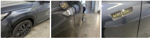
Door FL, Scratch(es), Repair and paint (complete)
