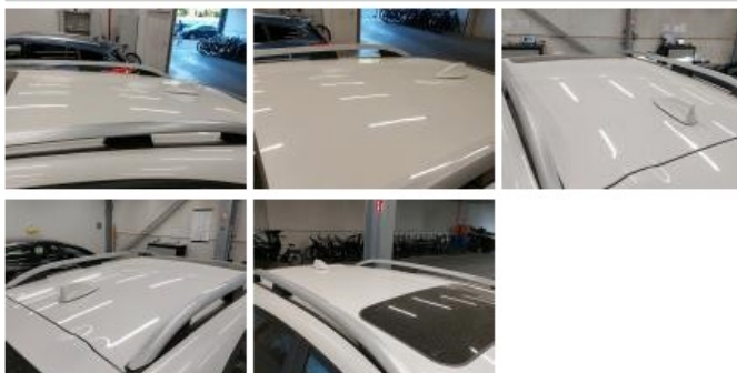
Roof, Hail damage, Repair and paint (complete)
