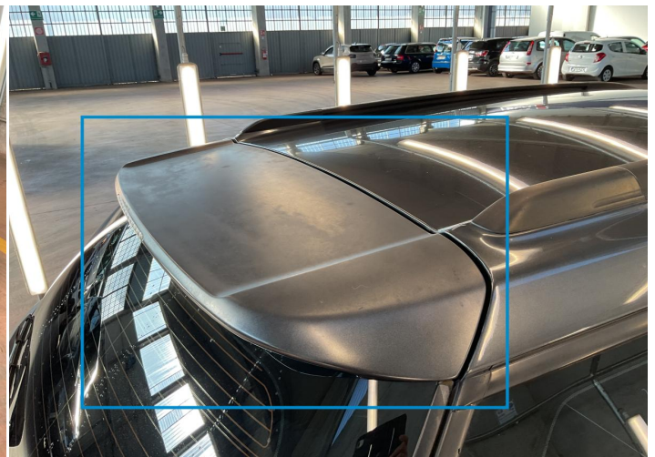
18. Spoiler / Back Paint / Poor Previous Repair -
