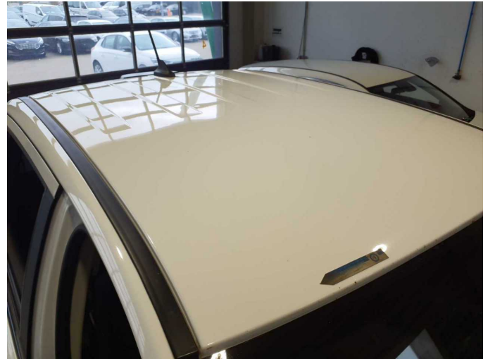
Damage 9: Roof: Roof (+ Dellen) - Corrosion - Repair and paint
