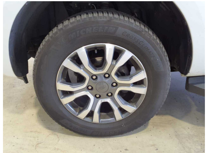
Wear and tear 7: Wheel / tyres: Alloy rim - front left side - Scratch(es) - No deduction
