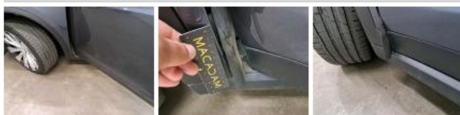
Wing trim FL, Damaged, Smart repair
