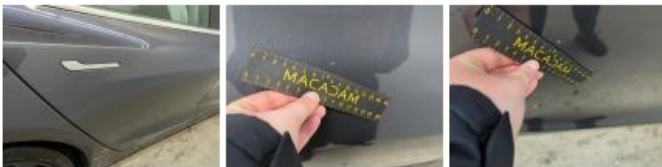
Door FR, Scratch(es), Repair and paint (complete)
