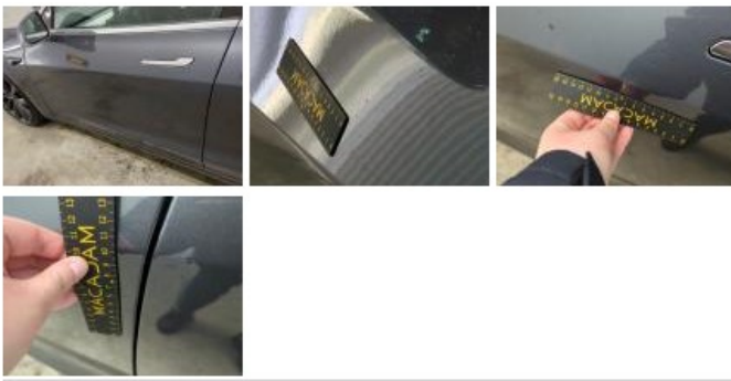
Door RL, Dent(s) and scratch(es), Repair and paint (complete)
