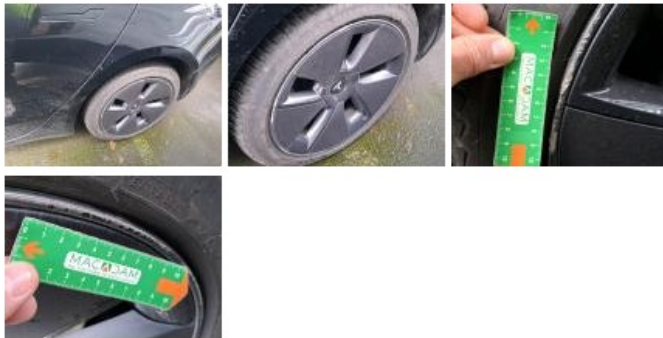
Alloy rim RR, Deformed / Strained, Replace
