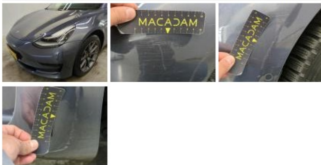
Bonnet, Chemical polution, Repair and paint (complete)
