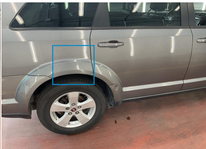
36. Fender / Back Right Bodywork / Dent -
