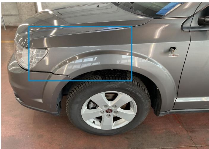
23. Fender / Front Left Paint / Chipping -
