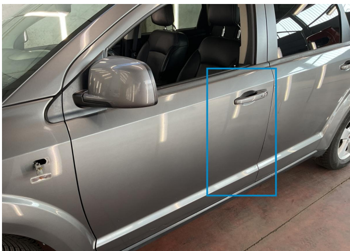
31. Door / Front Left Paint / Scratch / Line -
