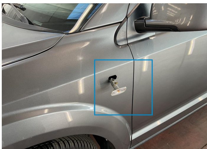
29. Wing Repeater / Left Bodywork / Breakage -
