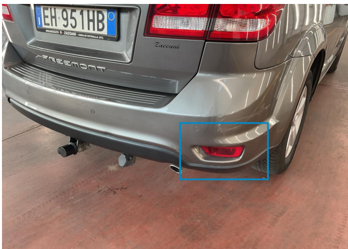
35. Fog Light / Back Right Bodywork / Breakage -
