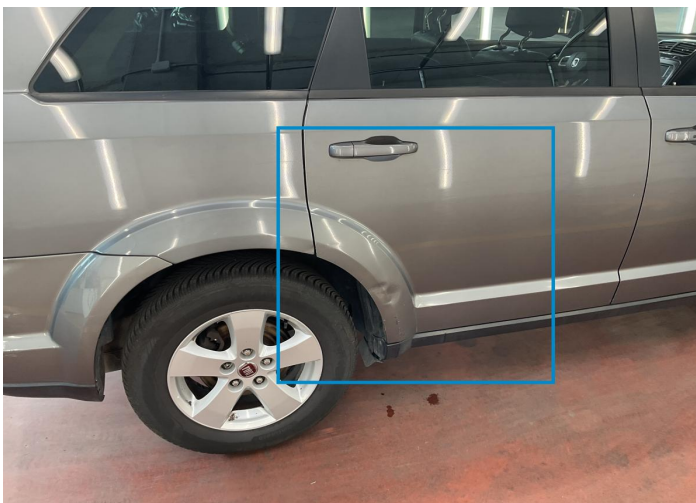
22. Door / Back Right Bodywork / Dent -
