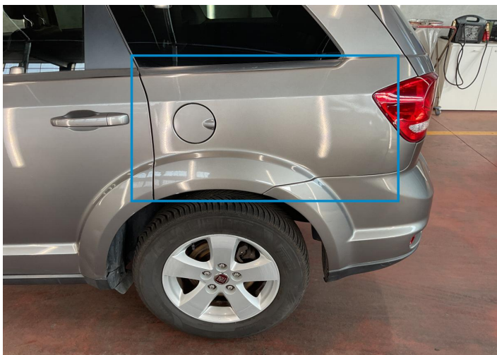
21. Fender / Back Left Bodywork / Dent -
