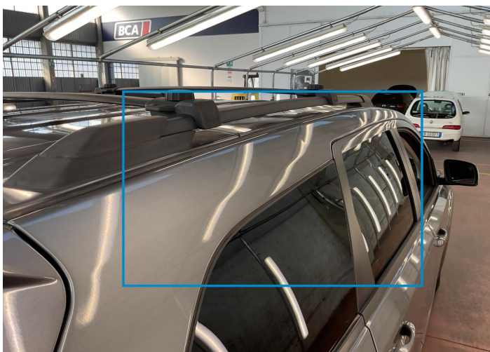
13. Pillar / Front Right Bodywork / Dent / Hail Area -
