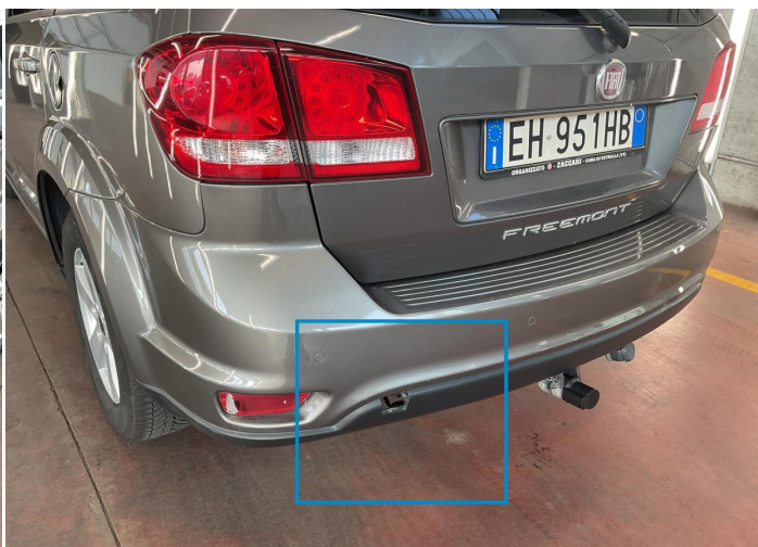
32. Towing Ring Hatches / Back Missing Part -
