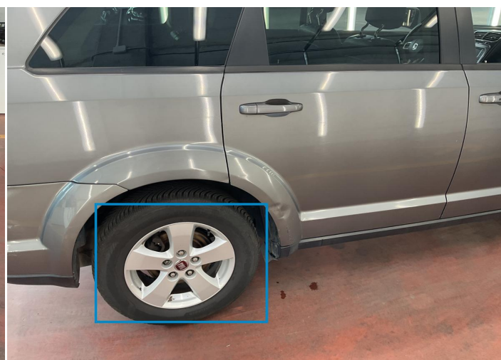
28. Rim / Back Right Out of Bodywork / Scratch -
