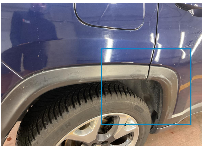
14. Fender / Back Right Bodywork / Dent -
