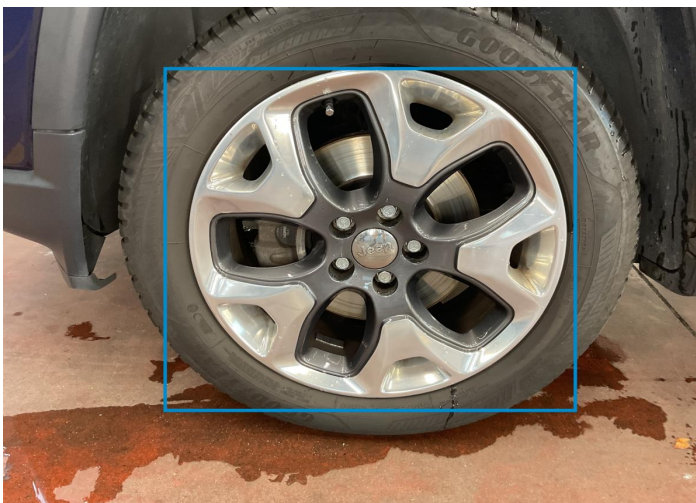
4. Rim / Front Left Out of Bodywork / Scratch -
