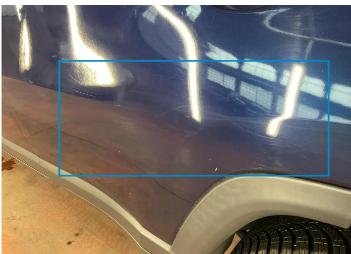
8. Door / Back Left Paint / Scratch / Line -
