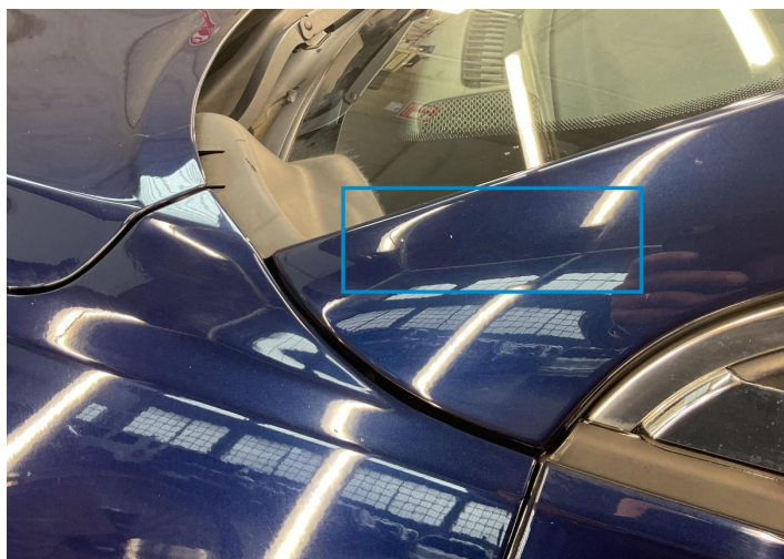
11. Pillar / Front Left Paint / Chipping -
