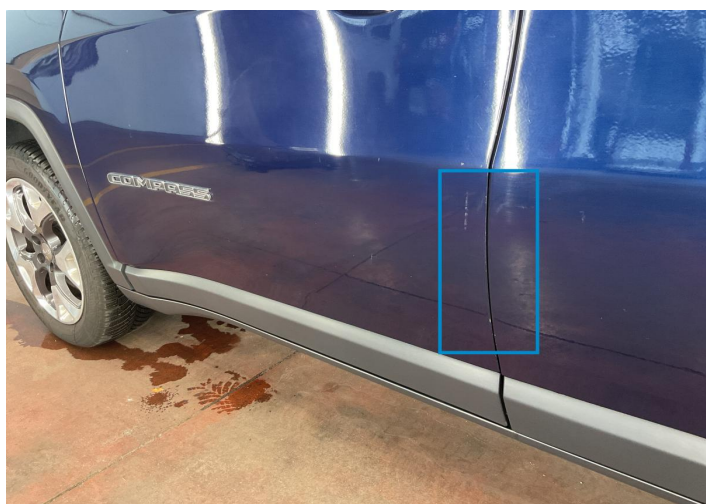
7. Door / Front Left Paint / Scratch / Line -
