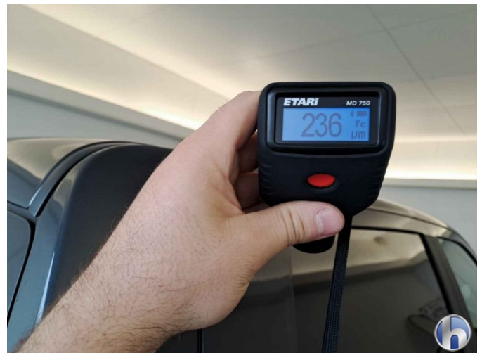
6. Roof frame - right
