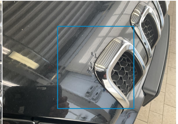
2. Hood Paint / Corrosion -
