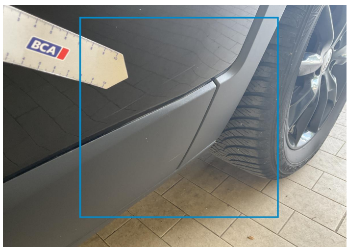
3. Door / Back Left Paint / Scratch / Scuff -
