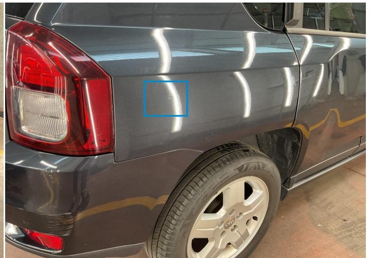
20. Fender / Back Right Bodywork / Dent -
