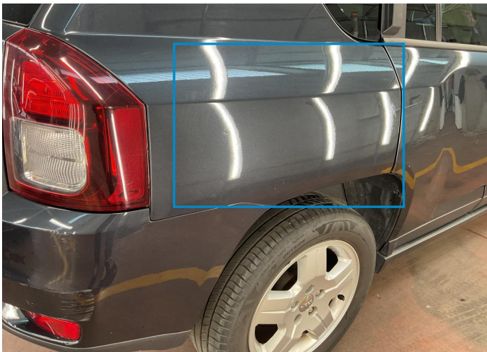
21. Fender / Back Right Bodywork / Poor Previous Repair -
