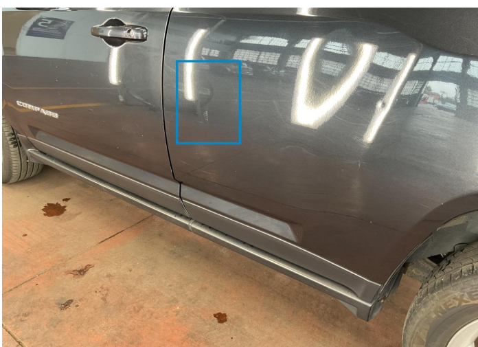
12. Door / Back Left Paint / Scratch / Line -
