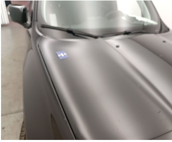
Front Bonnet // Painting-Chemical reaction
